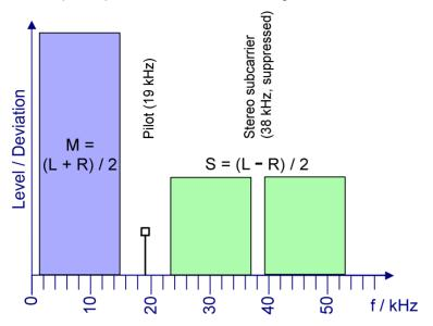
Fig. 4-56 Spectrum of the stereo MPX signal
