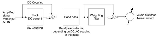
Fig. 4-47 Signal path for Multitone measurements
