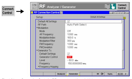
Fig. 4-31 Connection Control – RF generator settings (table)
