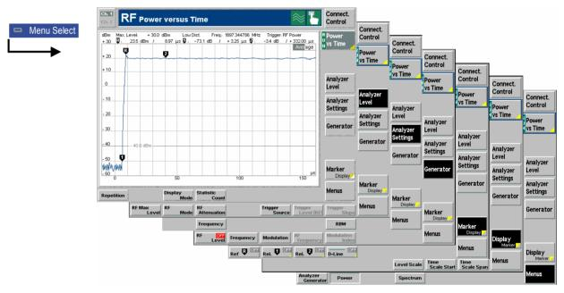
Fig. 4-22 Measurement menu Power
