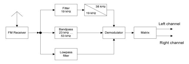
Fig. 4-55 Principle of the FM stereo decoder
