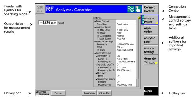
Fig. 3-2 Example of a measurement menu
