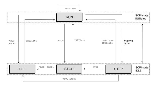
Fig. 5-7 Measurement states and control commands
