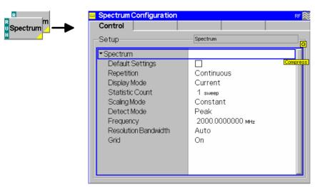
Fig. 4-27 Spectrum Configuration – Control
