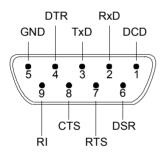
Fig. 8-2 Pin assignment of the RS-232-C interfaces
