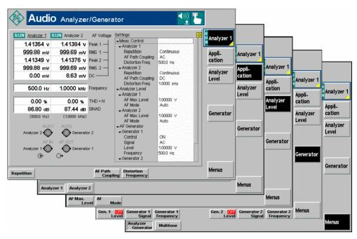
Fig. 4-36 Measurement menu Analyzer/Generator (Audio)
