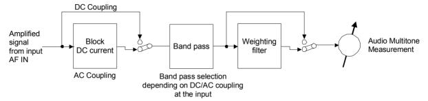
Fig. 51 Signal path for THD measurements
