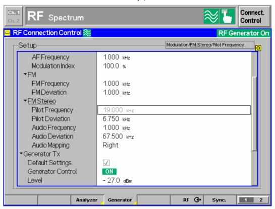
Fig. 4-57 Generator – FM Stereo configuration
