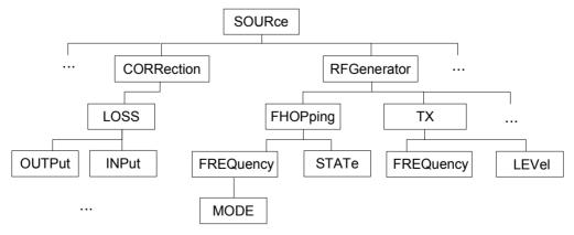
Fig. 5-2 Example for the tree structure of the SCPI command systems; the SOURce system
