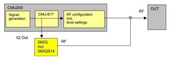
The CMU incl. option CMU-B17 in combination with R&S signal generator SMIQ incl. IQ fading simulator option SMIQB14 can be used for receiver Bit Error Rate tests under fading conditions. The IQ output of CMU-B17 transmitter (TX) path feeds the signal into SMIQ's IQ input. The SMIQ forwards the faded RF signal directly to the receiver (RX) of the DUT. The illustrated test setups depend on the test scenario selected on option CMU-B17.
