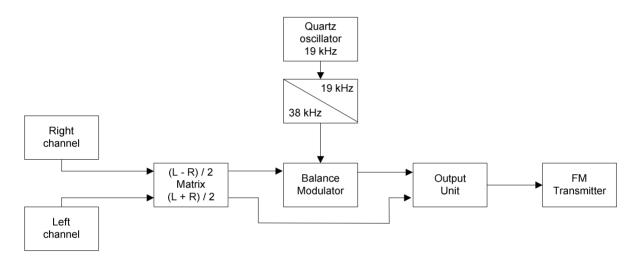
Fig. 4-54 Principle of the FM stereo coder
