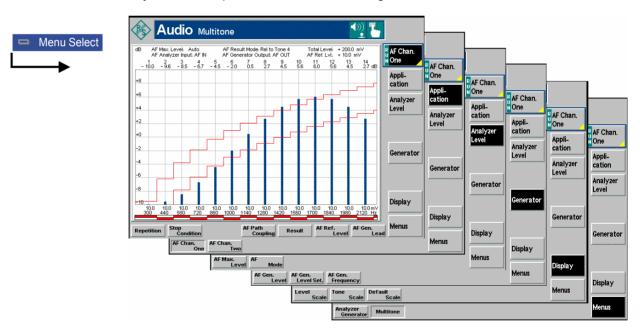
Fig. 4-42 Measurement menu Multitone
