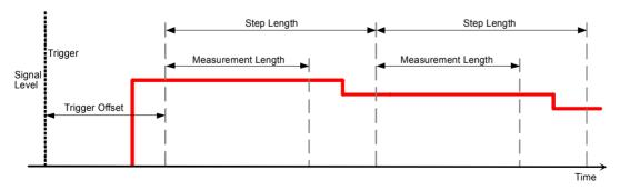
Figure 4-1 Step Length, Measurement Length and Trigger Offset
