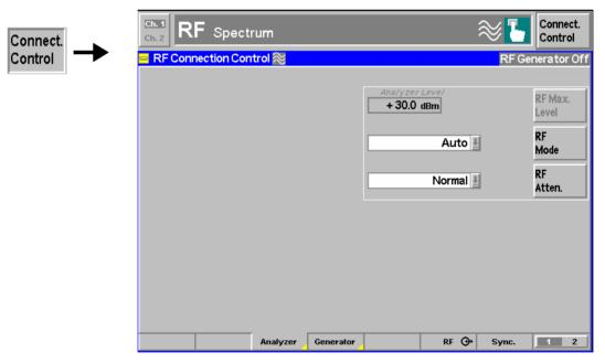
Fig. 4-28 Connection Control – RF analyzer settings (softkey)
