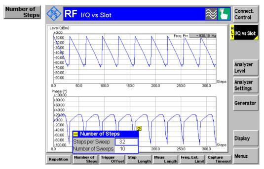
Figure 4-3 I/Q vs. Slot Number of Sweeps selection
