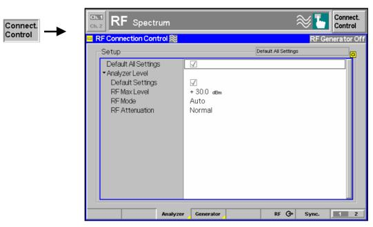
Fig. 4-29 Connection Control – RF analyzer settings (table)
