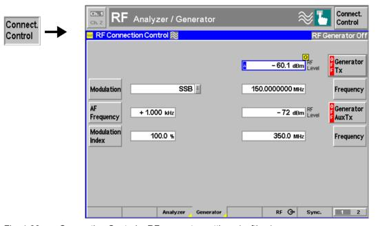
Fig. 4-30 Connection Control – RF generator settings (softkey)
