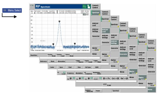
Fig. 4-25 Measurement menu Spectrum
