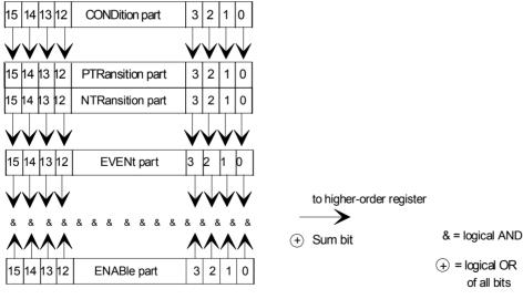
Fig. 5-4 The status register model
