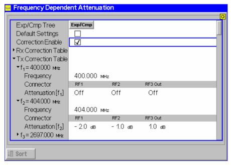
Fig. 4-1 Frequency-dependent attenuation
