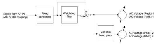
Fig. 4-40 AF analyzer input path configuration
