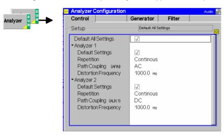
Fig. 4-38 Analyzer Configuration – Control
