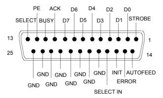
Fig. 8-5 Pin assignment of the LPT connector
