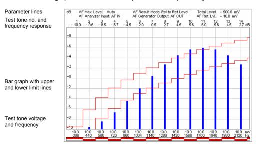
Fig. 4-43 Display of measurement results (Multitone)
