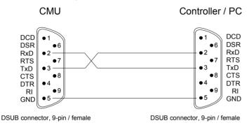
**CMU** Controller / PC DCD TxD DSR RxD RxD RTS RTS TxD CTS CTS DTR RI DSR **GND** GND DSUB connector, 9-pin / female DTR DCD ●22 RI 10 13
