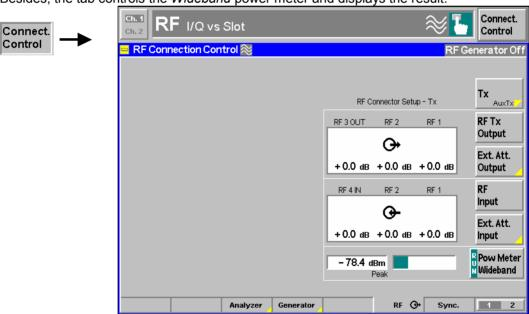
Fig. 4-32 Connection Control – RF connectors
