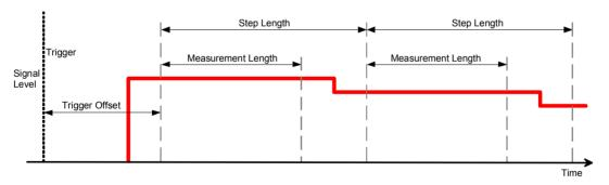
Figure 6-1 Step Length, Measurement Length and Trigger Offset
