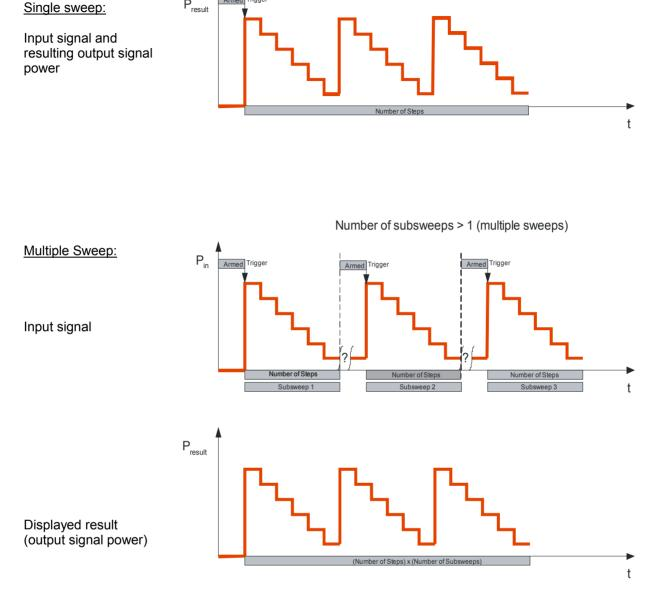
Figure 4-2: Input and output of single sweep and multiple sweep mode measurements
