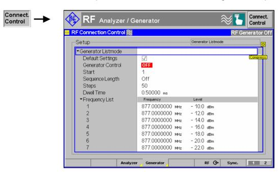
Figure 4-3 RF Configuration Control – Generator List Mode
