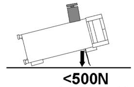
The instrument can be used in each of the positions shown here.
