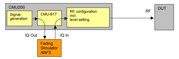
The CMU 200 incl. option CMU-B17 can be used in combination with the IQ fading simulator R&S ABFS for receiver tests under fading conditions. In this case the signal is routed to the DUT via the CMU's RF interface.
