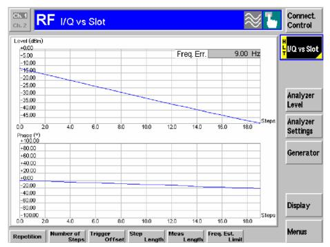
Figure 4-1 I/Q vs. Slot measurement menu
