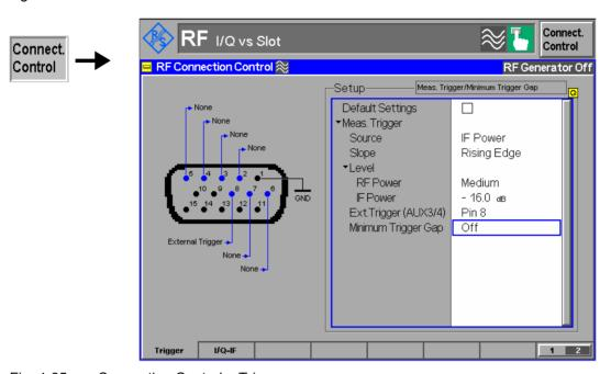
Fig. 4-35 Connection Control – Trigger
