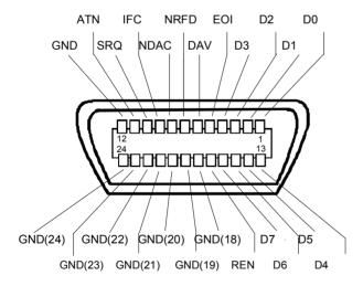
Fig. 8-1 Pin assignment of the GPIB bus interface
