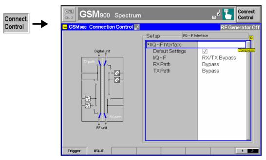
Fig. 4-4 Connection Control - I/Q-IF
