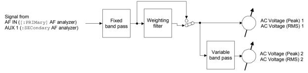
Fig. 6-1 AF analyzer input path configuration
